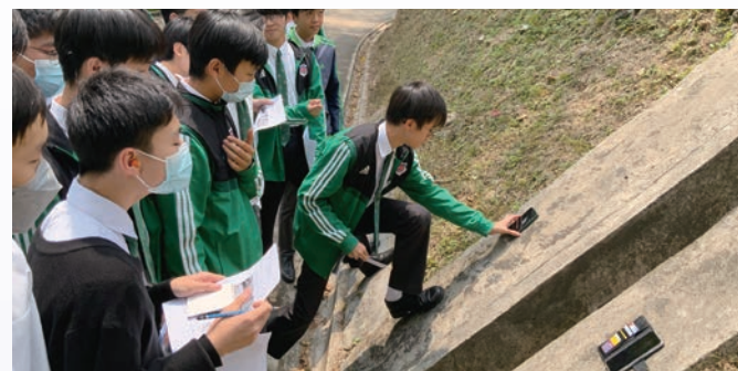
▲ Using mobile phones to measure inclination
