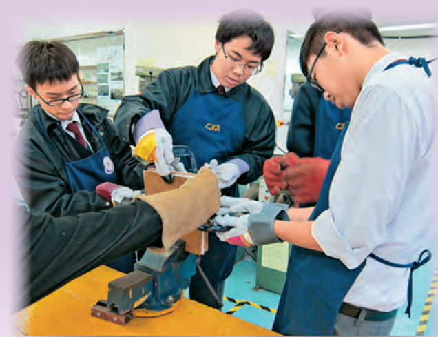
▲ Students are working collaboratively in moulding the acrylic sheet.
