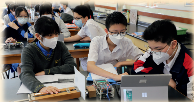
▲Students using mobile datalogger and sensor to measure the distance travelled and speed of a moving trolley.
